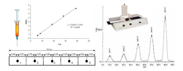
Results: Obtaining a correlation coefficient for the above measures as close to 1 (in absolute value), and the spatial coincidence of the peaks Rf in the radiochromatogram with the exact spots where the droplets were placed, provide the sufficient reliability for the radiochemical purity tests performed with that radiochromatograph.
